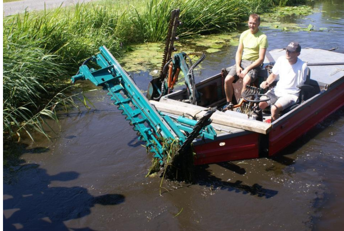
Figure 8.1: A weed cutting boat with adjustable mowing gear used for aquatic weed control in the Netherlands (Photo: R. Pot).
