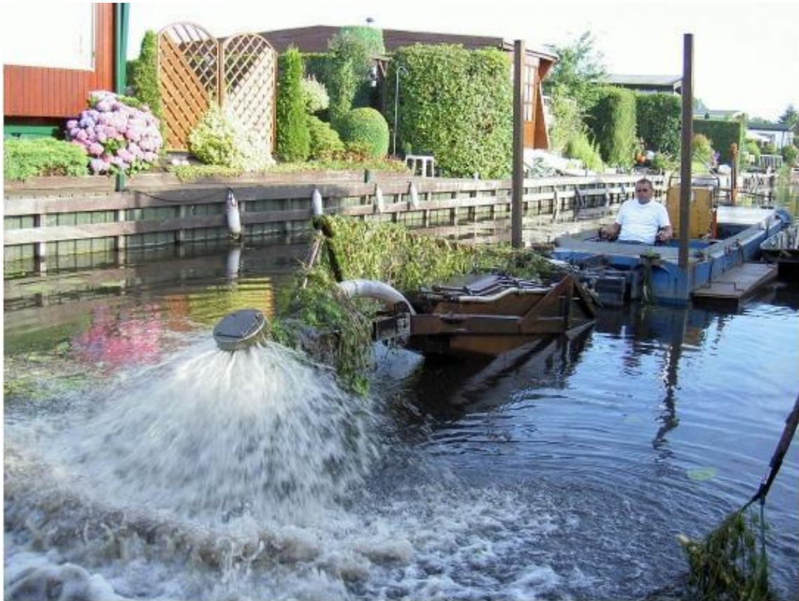
Figure 8.3: Application of the Hydro-venturi system. The head and water jet is raised above water to illustrate its operation (Photo: L. van Kersbergen).
