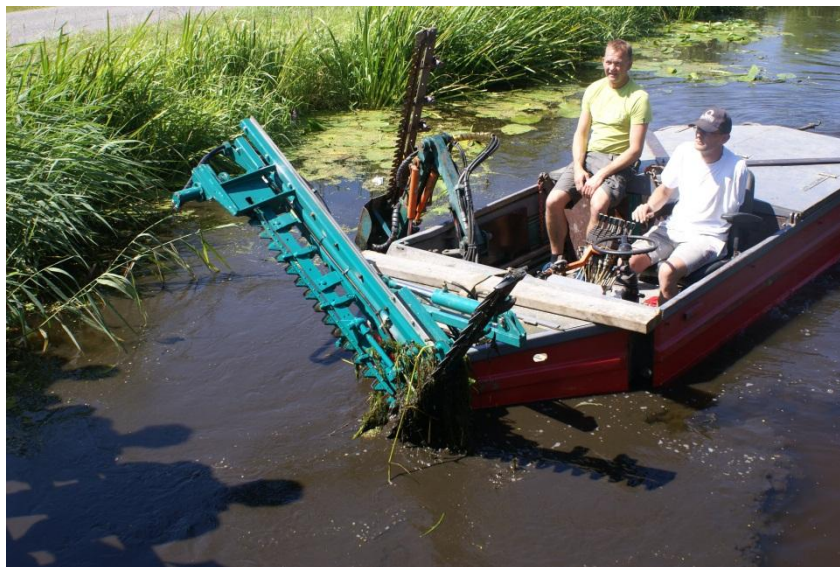
Figure 8.3: A weed cutting boat with adjustable mowing gear used for aquatic weed control in the Netherlands (Photo: R. Pot).
